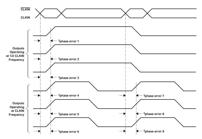
NOTES: A. Output skew,  $t_{Sk(0)}$ , is calculated as the greater of: - The difference between the fastest and slowest of  $t_{phase error n}$  (n = 1, 2, ... 6)
