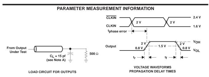
NOTES: A. Cl includes probe and jig capacitance.
