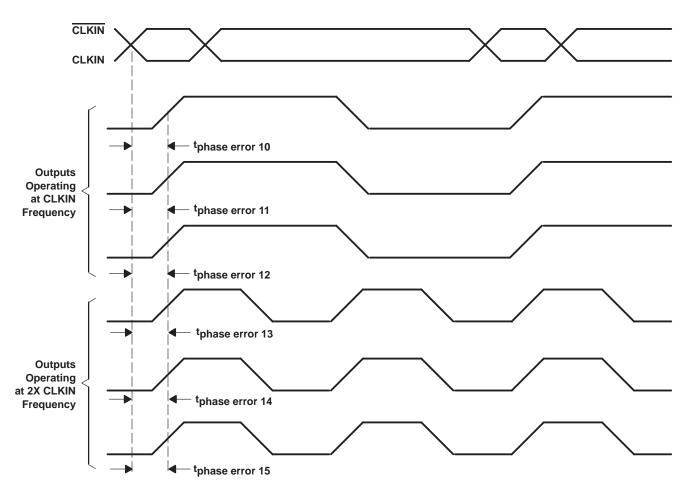
NOTES: A. Output skew,  $t_{sk(0)}$ , is calculated as the greater of: - The difference between the fastest and slowest of  $t_{phase \ error \ n}$  (n = 10, 11, . . . 15)
