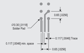
Trace width/spacing for non-solder mask defined = 0.1167 [.0046] Trace width/spacing for solder mask defined with  $\emptyset$ 0.33 solder pad = 0.0733 [.0029]
