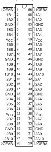
The 74ACT16861 is packaged in TI's shrink small-outline package, which provides twice the I/O pin count and functionality of standard small-outline packages in the same printed-circuit-board area.
