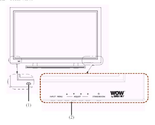
(1) Remote control window: The window with a power indicator and IR receiving sensor are used for indicating power status and receiving remote control signals.
