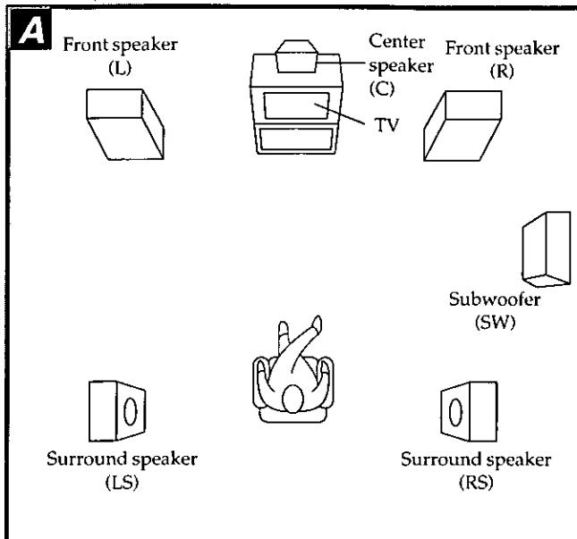
To enjoy discrete multi-channel sound reproduction using this unit, read through the instructions given below before installing the speakers. **A**
