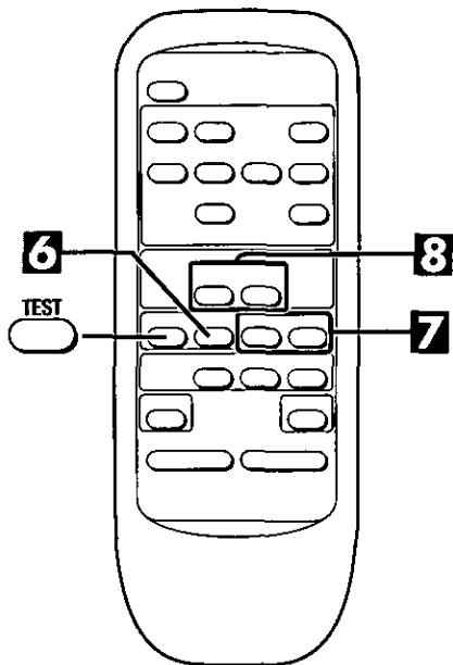
**6 Press LEVEL to select speakers to adjust the output level.**
