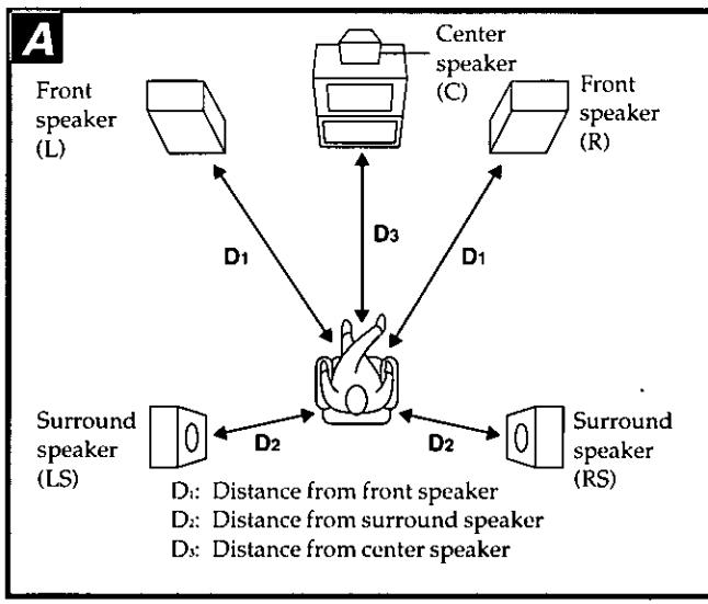
By adjusting the delay time, the difference in the distance from the viewing and listening position to the front speakers and the distance to the center speaker and surround speakers can be offset and made equal. This achieves better sound localization and makes a more life-like reproduction of the sound field possible.
