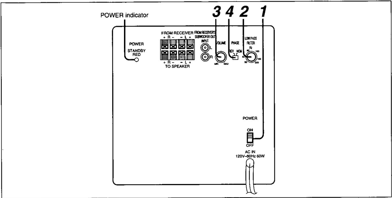
Set the low pass filter, volume and phase to suit characteristics of the front speaker and subwoofer combination.
