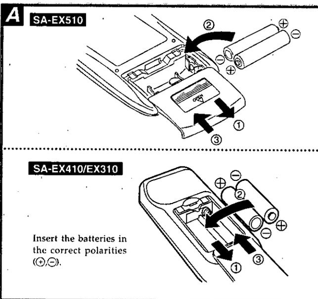
Insert the batteries in the correct polarities (+, -).
