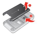
• Remove the battery cover and insert the memory card with the goldcoloured contacts facing down.
