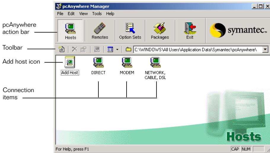
The buttons on the pcAnywhere action bar let you switch between host and remote modes, view and edit properties of global options and packages, and exit pcAnywhere.
