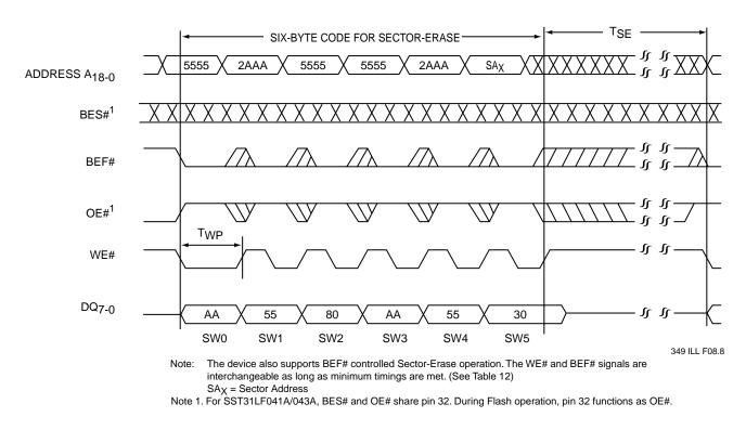
FIGURE 10: WE# CONTROLLED FLASH SECTOR-ERASE TIMING DIAGRAM
