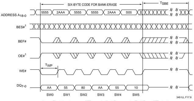
Note: The device also supports BEF# controlled Bank-Erase operation. The WE# and BEF# signals are interchangeable as long as minimum timings are met. (See Table 12)
