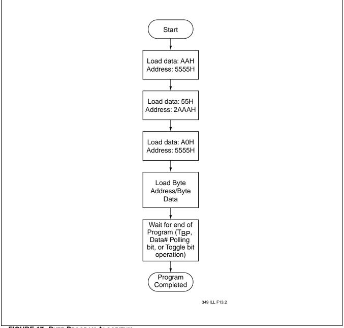
FIGURE 17: BYTE-PROGRAM ALGORITHM
