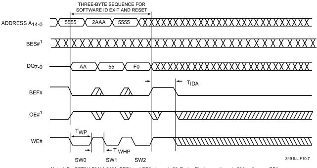
Note 1. For SST31LF041A/043A, BES# and OE# share pin 32. During Flash operation, pin 32 functions as OE#.
