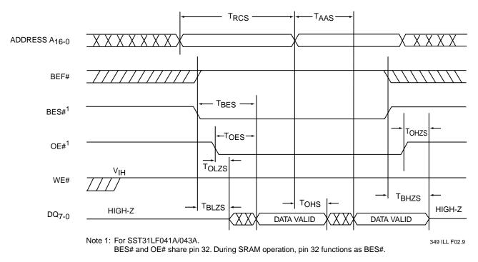
FIGURE 3: SRAM READ CYCLE TIMING DIAGRAM
