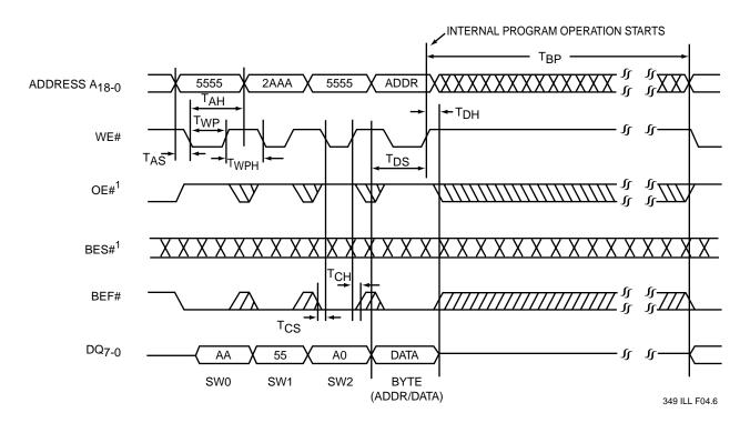
Note 1. For SST31LF041A/043A, BES# and OE# share pin 32. During Flash operation, pin 32 functions as OE#.
