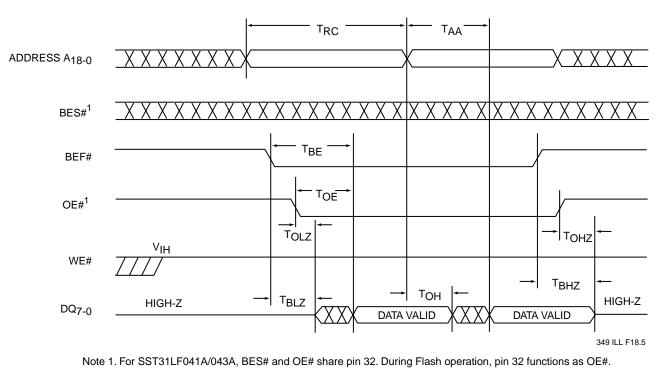
FIGURE 5: FLASH READ CYCLE TIMING DIAGRAM
