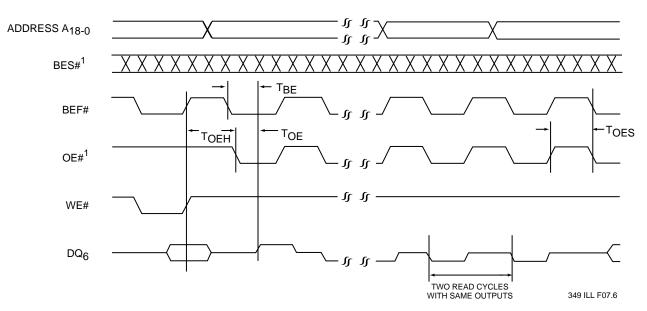
Note 1. For SST31LF041A/043A, BES# and OE# share pin 32. During Flash operation, pin 32 functions as OE#.
