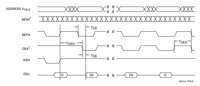
Note 1. For SST31LF041A/043A, BES# and OE# share pin 32. During Flash operation, pin 32 functions as OE#.
