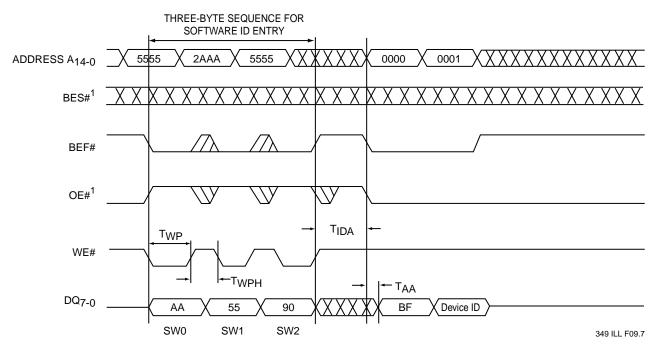
Note 1. For SST31LF041A/043A, BES# and OE# share pin 32. During Flash operation, pin 32 functions as OE#. Note: Device ID = 16H for SST31LF041A, 17H for SST31LF041, 65H for SST31LF043 and 66H for SST31LF043A.
