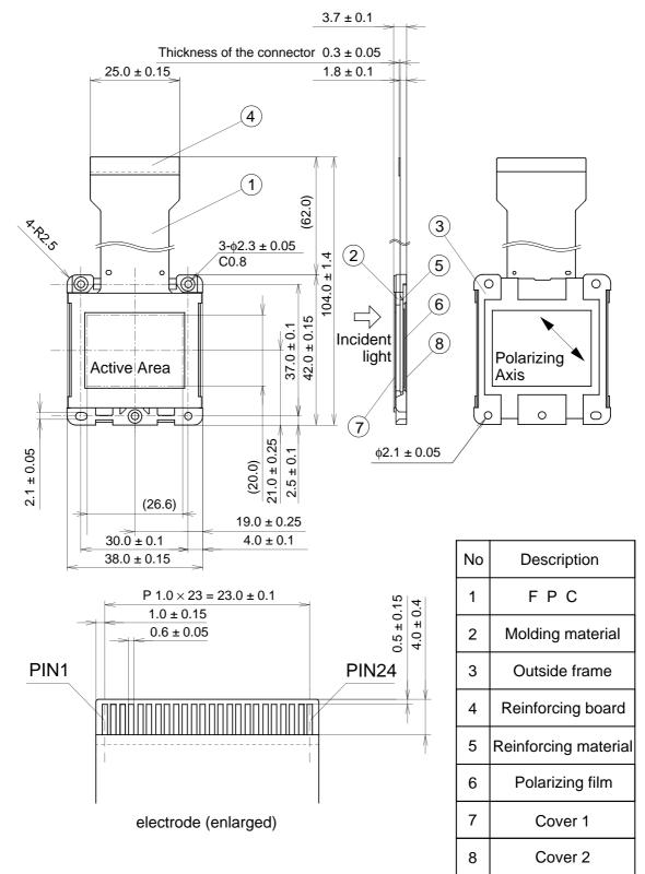
The rotation angle of the active area relative to H and V is  $\pm 1^{\circ}$ .
