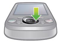
• Press the navigation key upwards, downwards, left or right to move through the menus.
