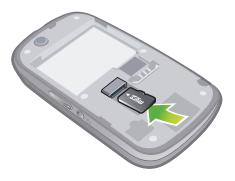
• Remove the battery cover and insert the memory card with the gold-coloured contacts facing down.
