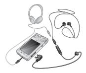
You can connect both a handsfree and headphones with a 3.5 mm (0.14 inch) plug to the phone. They can be connected to the phone at the same time.
