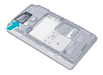
• Remove the battery cover and insert the memory card with the gold-colored contacts facing down.
