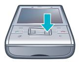
• Press the navigation key upwards, downwards, left or right to move through the menus.
