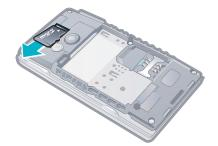
• Remove the battery cover and slide the memory card to remove it.
