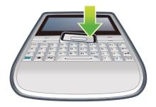
• Press the navigation key upwards, downwards, left or right to move around the screen. Press the selection key (at the center of the navigation key) to select an item.
