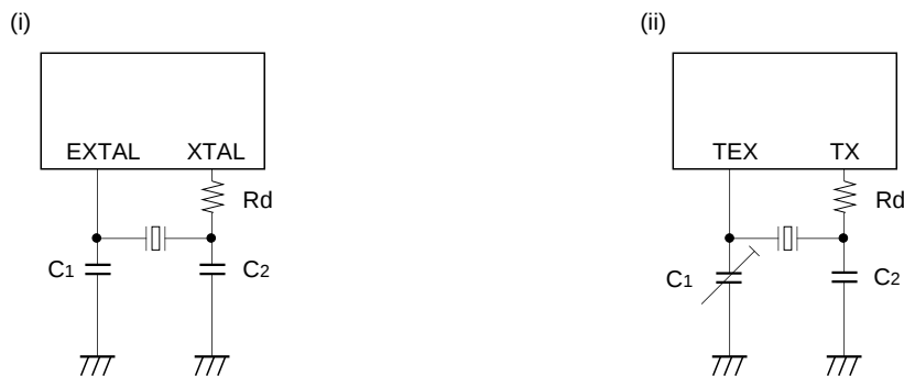
Fig. 11. Recommended oscillation circuit
