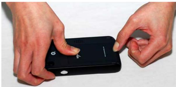
2. Place the included battery into the battery compartment, so that the battery's bar code label is face up, near the bottom of the device.
