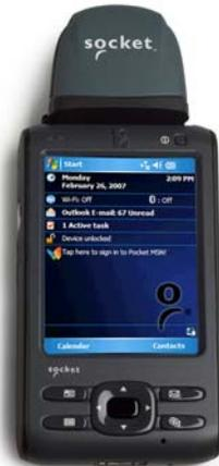
2. When SocketScan is running, a SocketScan icon will appear at the bottom of the Today screen. Make sure the appropriate icon appears to indicate that your device is ready to collect data.
