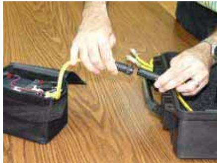
**Figure 1-44 - Disconnecting the batteries**
