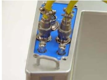
**Fig. 1-27 Close-up of the Battery leads connected in P1 and P2**
