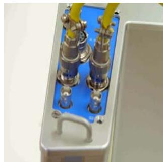
**Fig. 1-16 Close-up of the Battery leads connected in P1 and P2**
