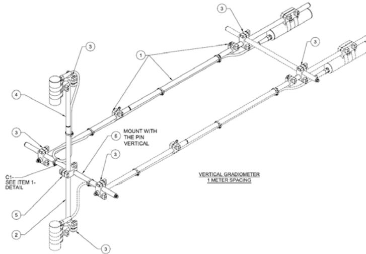
**Figure 1-36 - 1.0 m Vertical Gradient Configuration**
