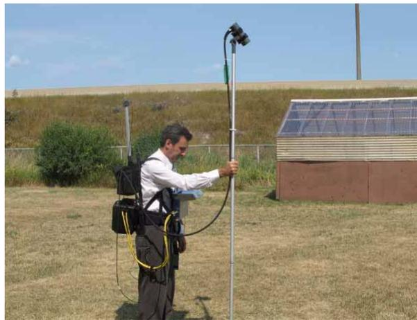
**Figure 1-40 - Stop and Go Configuration**
