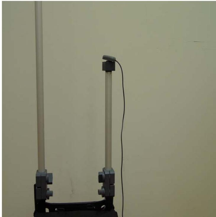
**Figure 3-2 - Mounting the Internal GPS antenna**
