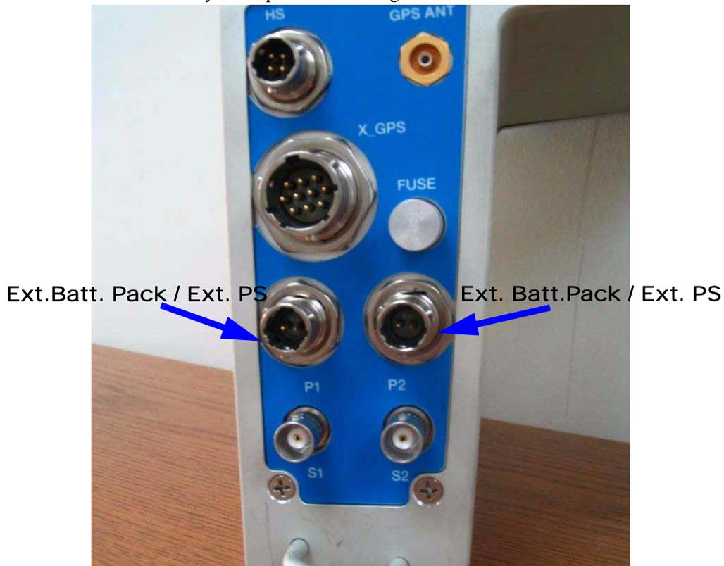
**Figure 1-42 - Location of External Battery Pack Connectors**
