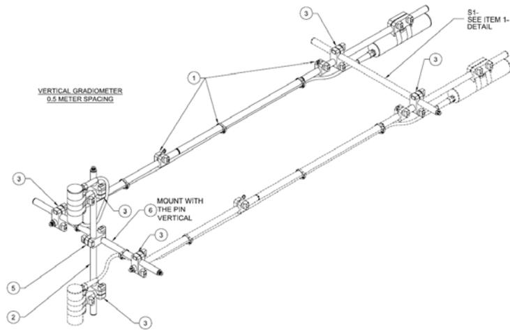
**Figure 1-34 - 0.5 m Vertical Gradient Configuration**
