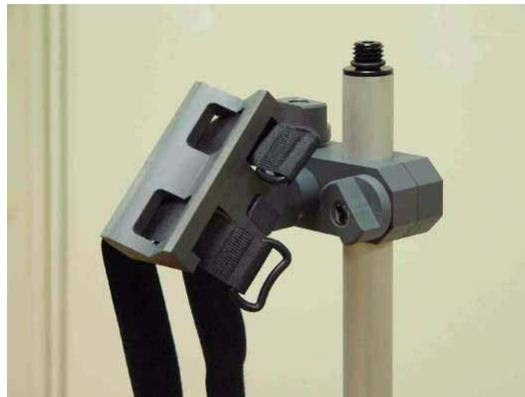
Figure 1-21 - Close-up of the sensor clamp assembled in the sensor pole
