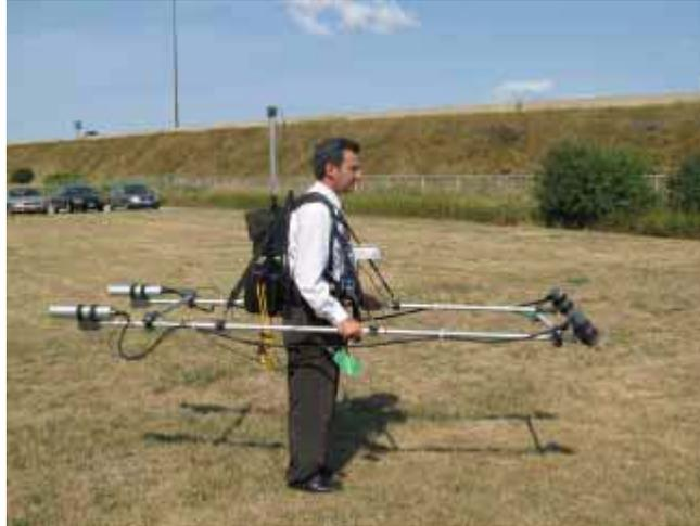
**Figure 1-38 - Example of Horizontal Gradient Set Up**
