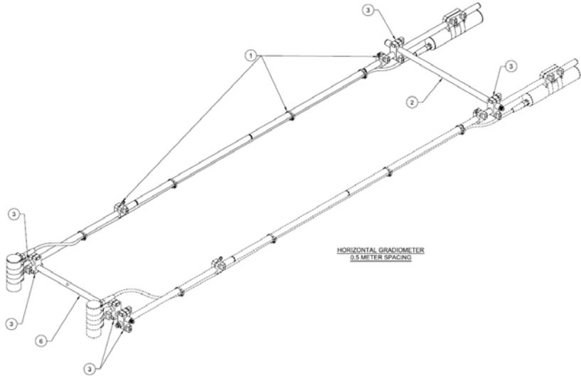
Figure 1-35 - 0.5 m Horizontal Gradient Configuration
