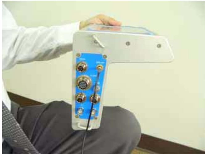
**Figure 1-29 - Internal GPS antenna connection**
