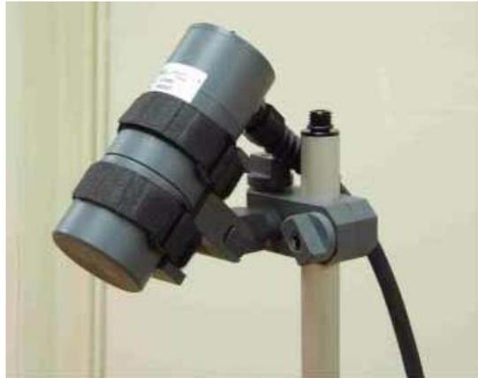
**Figure 1-22 - Close-up of the sensor mounted to the sensor clamp**
