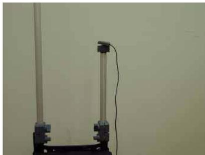
**Figure 1-30 - Mounting the Internal GPS antenna**
