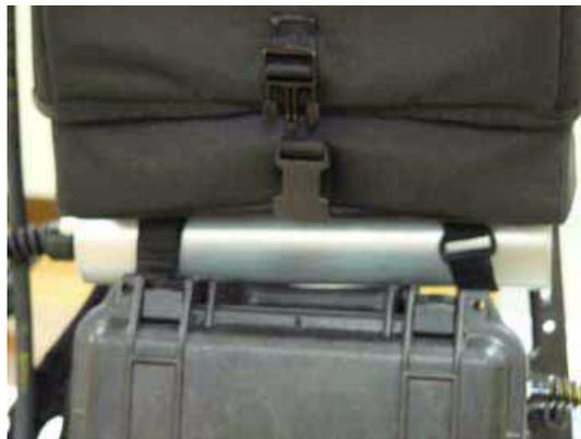
**Figure 1-23 - Close-up of the sensor electronics mounted on the Back-pack**
