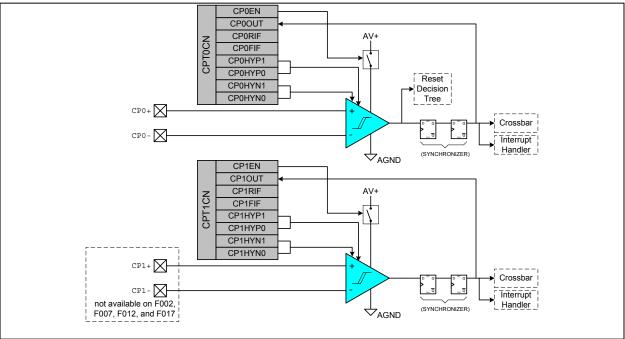
Figure 8.1. Comparator Functional Block Diagram
