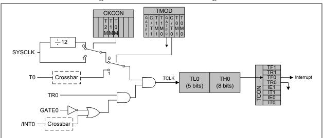
Figure 19.1. T0 Mode 0 Block Diagram
