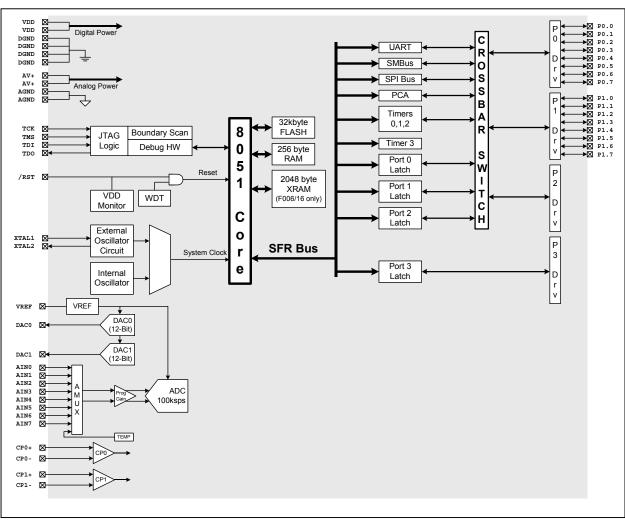
Figure 1.2. C8051F001/06/11/16 Block Diagram
