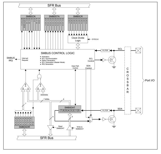
Figure 16.1. SMBus Block Diagram
