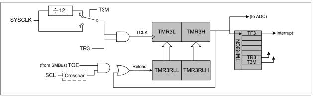
Figure 19.20. TMR3CN: Timer 3 Control Register
