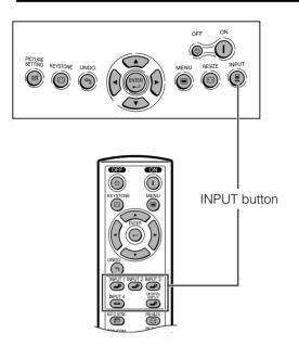
Press **INPUT** on the projector, **INPUT 1**, **INPUT 2**, **INPUT 3**, **INPUT 4** or **DIGITAL INPUT** on the remote control to select the desired input mode.
