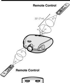
The remote control can be used to control the projector within the range shown on the left.
