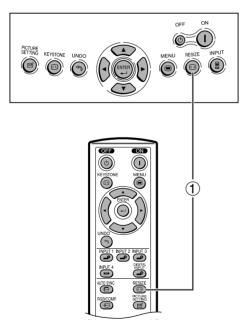
This function allows you to modify or customize the picture display mode to enhance the input image. Depending on the input signal, you can choose NORMAL, BORDER or STRETCH image.
