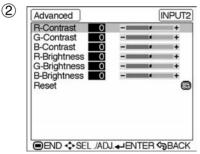
Detailed picture adjustments can be made in addition to the adjustments on the normal menu screen.
