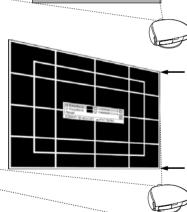
(3) Align the edge of the screen closest to the projector with the test pattern by adjusting the zoom and the Swivel Stand. (See pages 16 and 17.)
