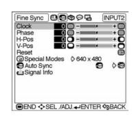
When displaying computer patterns which are very detailed (tiling, vertical stripes, etc.), interference may occur between the DMD pixels, causing flickering, vertical stripes, or contrast irregularities in portions of the screen. Should this occur, adjust "Clock", "Phase", "H-Pos" and "V-Pos" for the optimum computer image.
