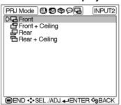
This projector is equipped with a reverse/invert image function which allows you to reverse or invert the projected image for various applications.
