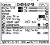
When no input signal is detected for more than 15 minutes, the projector will automatically shut off. The on-screen message on the left will appear five minutes before the power is automatically turned off.
