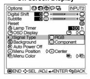
This function allows you to select the input signal type Component or RGB for INPUT 2.
