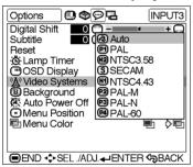
The video input system mode is preset to "Auto"; however, it can be changed to a specific system mode if the selected system mode is not compatible with the connected audiovisual equipment.
