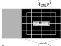
(1) Project the test pattern of the Keystone correction function onto the screen. Rotate the Focus ring until the image on the screen becomes clear. (See page 16.)
