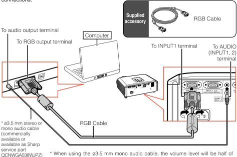
\* When using the ø3.5 mm mono audio cable, the volume level will be half of when using the ø3.5 mm stereo audio cable.
