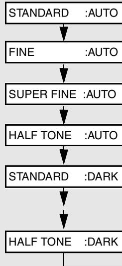
**Note:** In order to transmit in SUPER FINE resolution, the receiving fax machine must also have that resolution. If it doesn't, your machine will automatically step down to the next best available setting.
