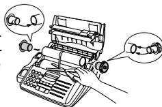
5. Pull the empty spool toward the back of the compartment, unwinding the leader from the spool with film. Insert the empty spool into the compartment so that the gear and spool fit into the slots on each side of the compartment.
