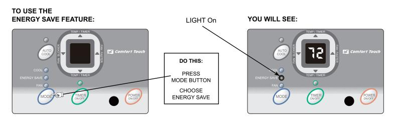
**Note:** In this mode, the fan will continue to run for another 3 minutes after the compressor shuts off. The fan then cycles on for 2 minutes at 10 minute intervals until the room temperature is above the set temperature, at which time the cooling system turns back on.
