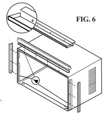
2. Install top angle and side retainers to cabinet as shown in FIG. 6.
