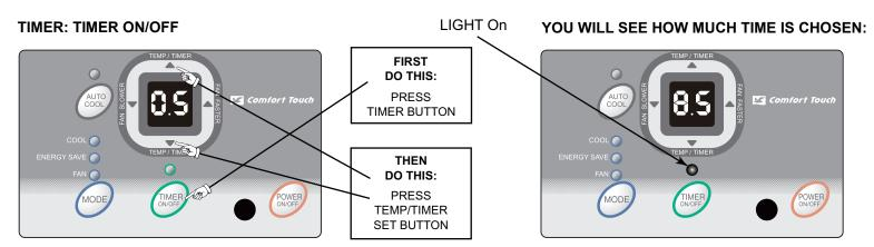
**Note 1:** For Timer Off, the unit must be in the On position. **Note 2:** For Timer On, the unit must be in the Off position.
