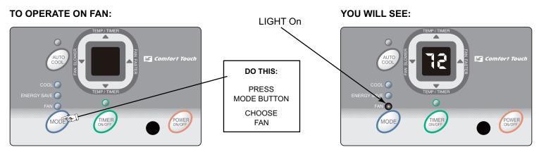
**Note:** Use this function only when cooling is not desired, such as for room air circulation or to exhaust stale air. (Remember to open the vent during this function, but keep it closed during cooling for maximum cooling efficiency.) You can choose any fan speed you prefer. (Except "Auto Cool").
