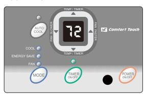
**Note:** Tap or hold either up ( $\triangle$ ) or down ( $\nabla$ ) button until the desired temperature is seen on the display. This temperature will be automatically maintained anywhere between 60°F (16°C) and 90°F (32°C) for cooling mode. If you want the display to read the actual room temperature. See "To Operate on Fan" section on Page 13.
