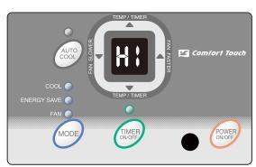
Press the Fan Faster button will increase the fan speed from Low (LO), to Medium (ME), to High (HI). The digital display will indicate your chosen speed. Press the Fan Slower button will decrease the fan speed from High (HI), to Medium (ME), to Low (LO). The digital display will indicate your chosen speed. After 5 seconds the display will revert back to the set temperature.
