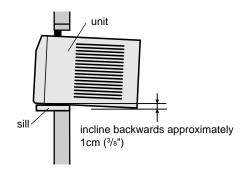
Insert the bottom gasket into the space between the window sill and the bottom of the unit to seal outside air.
