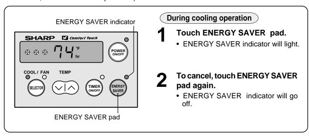
**NOTE:** ENERGY SAVER cannot be set during fan only (HIGH FAN, MED FAN, LOW FAN) operation.
