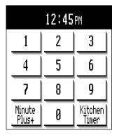
The Home Page is the beginning. It shows the time of day, if the clock has been set. It also shows Minute Plus +, where by touching the screen the next screen appears, making it easy to select one of twelve commonly used times. Touching Kitchen Timer tells the oven that the time set is only for timing, not for cooking.
