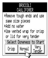
2 Touch the desired doneness, and the oven will start automatically. When the sensor detects the vapor emitted from the food, remaining cooking time will appear. The oven door can be opened whenever the count down time is displayed on the Touch Screen.
