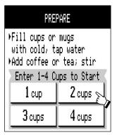
2 Touch desired number on the screen. The oven will start automatically.
