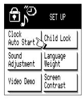
1 Press Set Up pad and then touch the desired function: Clock/Auto Start.
