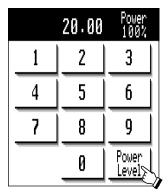
**4** Enter cooking time, 2, 0, 0, 0 by using numbers on the screen. Touch Power Level.
