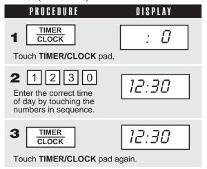
This is a 12 hour clock. If you attempt to enter an incorrect clock time, *ERRUR* will appear in the display. Touch the **STOP/CLEAR** pad and re-enter the time.
