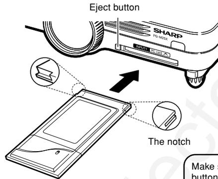
Make sure that the Eject button is not out, and that the notch on the card is to the left, when installing the card.
