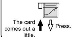
Remove the card from the slot and store it in a safe place. If the Eject button is out, press it once more to set it back in place.
