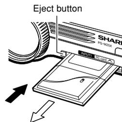
**1** Press the Eject button. The Eject button pops out.
