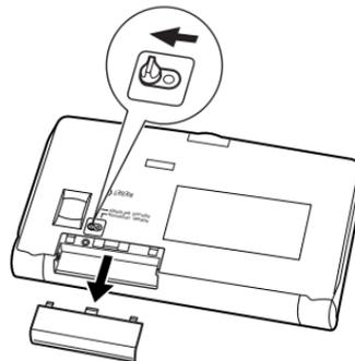
4. Remove the old batteries by pulling the ribbon tab.
