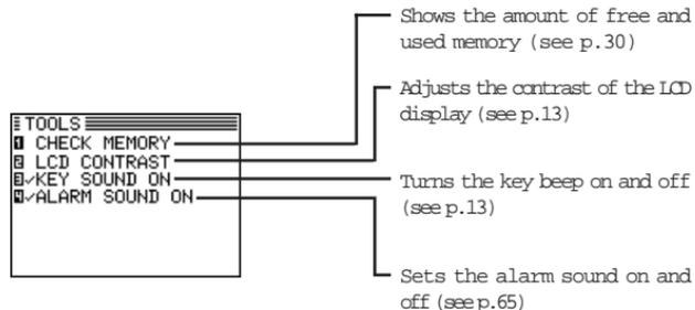
Other important facilities and functions are provided via the PREFERENCES menu, which allows you to tailor the Organizer and is described in Chapter 10, and the PERIPHERALS menu, which provides commands for data transferring, described in Chapter 9.
