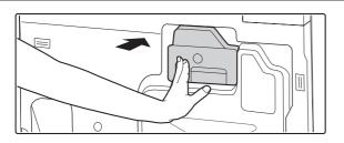
Push the cartridge in until it locks securely in place.
