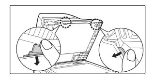
Open the holders on the automatic document feeder that hold the original pressure sheet.
