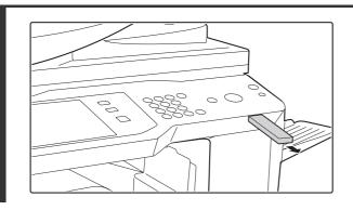
Remove the USB memory device from the machine.
