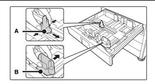
Adjust the guide plates A and B by squeezing their lock levers and sliding them to match the vertical and horizontal dimensions of the paper to be loaded.
