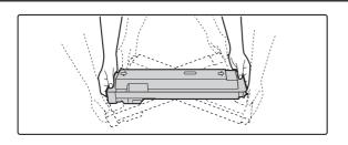
Remove the new toner cartridge from its packaging and shake it 5 or 6 times as shown.
