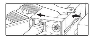
While pulling the lever, slide the saddle stitch finisher to the left until it stops.
