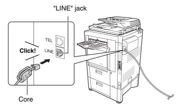
Insert the end of the cord with the core into the "LINE" jack.
