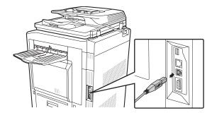
(3) Connect the other end of the cable to the USB connector (A type) on your computer.
