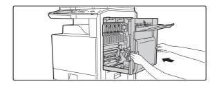
Return the lever to the normal position when finished feeding envelopes.
