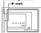
All originals should be placed in the left center position. Align the middle of the original with the tip of the ▶ mark.
