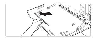
Remove the cleaning tool for the writing unit from the front cover.
