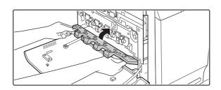
Close the main charger cover and rotate the lock levers in the direction of the arrows to lock the cover.
