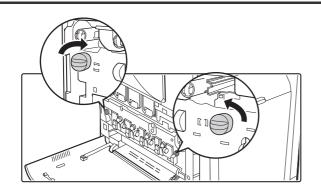
Close the main charger cover and rotate the lock levers in the direction of the arrows to lock the cover.
