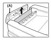
Open A section's cover and remove misfeed originals.
