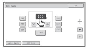
Touch a numeric value display key to directly enter a value with the numeric keys.
