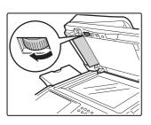
Open the automatic document feeder and remove misfeed originals while rotating the transfer roller in the direction of the arrow.
