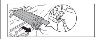
Hold down the lever on the drum cartridge with your finger and pull the drum cartridge toward you.
