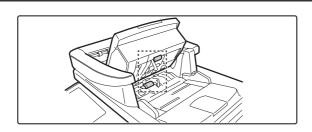
To clean the removed rollers, wipe each roller with a clean cloth.
