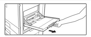
When loading paper larger than 8-1/2" x 11" or A4, be sure to pull out the bypass tray extension. Pull the bypass tray extension all the way out. If the bypass tray extension is not pulled all the way out, the size of the loaded paper will not be correctly displayed.
