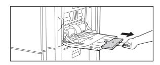
When loading paper larger than 8-1/2" x 11"R or A4R, be sure to pull out the bypass tray extension. Pull the bypass tray extension all the way out. If the bypass tray extension is not pulled all the way out, the size of the loaded paper will not be correctly displayed.
