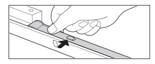
(3) Fit the holder into the hole in the tip (the end with the cleaner) of the cleaning tool.
