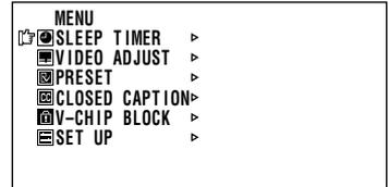
**2** Press **▲/▼** to move the cursor to V-CHIP BLOCK, and press **◀/▶** to enter.
