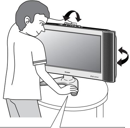
Hold the carrying handle and tilt the screen while steadying the stand with your other hand. You can adjust the screen vertically up to 5 degrees forward or 10 degrees backward, or rotate 25 degrees horizontally.
