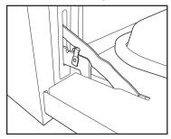
Lock engaged for door removal.
