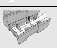
**3** Squeeze the paper guide and pull up to move it to the appropriate holes for the length of the paper. Push the guide down into the holes.
