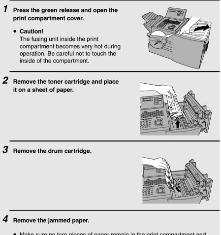
• Make sure no torn pieces of paper remain in the print compartment and rollers.
