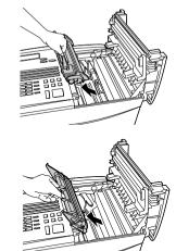
**4** Open the black cover (hinged on the left) at the bottom of the compartment. If jammed paper is visible, remove it.
