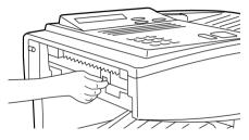
**3** Insert the new ink cartridge into the machine (make sure that the tab is facing out).
