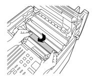
**3** If the jammed paper isn't visible, remove the toner cartridge and then the drum cartridge.
