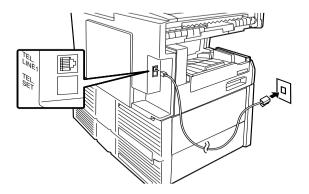
**Note:** The fax machine is set for touch-tone dialing. If you are on a pulse dial (rotary) line, you must set the fax machine for pulse dialing by changing Option Setting 22. This procedure is described in Chapter 6, *Optional Settings*.
