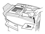
Note: When inserting a large number of pages in the feeder, slant the front end of the stack so that the bottom pages enter first.
