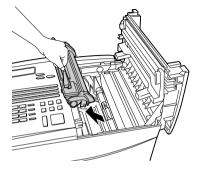
**3** If you are replacing the drum cartridge, remove the old cartridge and dispose of it according to local regulations.
