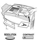
**3** If you pressed the **SPEAKER** key, dial the number of the receiving machine by pressing the numeric keys on the fax machine.
