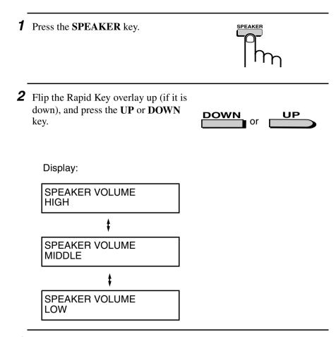
**3** When the display shows the desired volume level, press the **SPEAKER** key to turn off the speaker.
