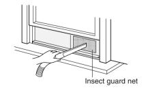
The cooling performance may be reduced or stop completely if the insect guard net becomes clogged with dust.
