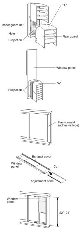
If the inner height of the window is between 24" (609mm) and 36.8" (934mm) inclusive.
