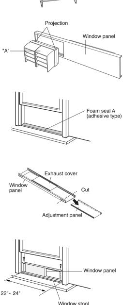
If the inner width of the window is between 24" (609mm) and 36.8" (934mm) inclusive.
