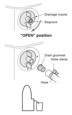
If draining of the water is not desirable, install the exhaust hose (See Page 16), turn the drainage nozzle to the CLOSE position, and check that the drainage nozzle is covered with the stopcock. In this operation, the water tank inside the unit may be full, the unit stops operating and then the TIMER, OPERATION and MEGA COOL lamps are blinking, depending on room condition. In this case, drain out the water within the unit (See Page 29).
