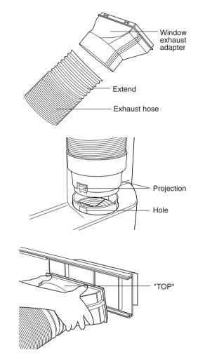
The exhaust hose should be as short as possible for operational efficiency; however, it must not be twisted or bent.
