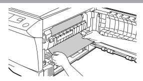
Raise the fusing unit release lever and then close the side cover by pressing the round projections near the side cover open button. The misfeed (8/v) indicator will go out and the ready ((\*)) indicator will light up.
