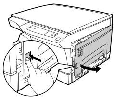
Remove the CAUTION tape from the front cover and remove the two protective pins from the fusing unit by pulling the strings upward one at a time.
