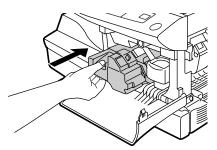
Close the front cover and then the side cover by pressing the round projections near the side cover open button.
