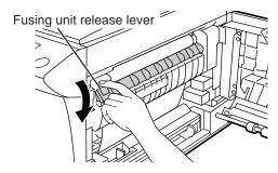
Gently remove the misfed paper from under the fusing unit as shown in the illustration. If the paper cannot be removed, proceed to "C Misfeed in the transport area".
