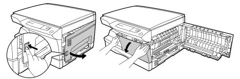
**2** Gently pull the TD cartridge out while pressing the lock release button. Dispose of the old TD cartridge in accordance with local regulations.
