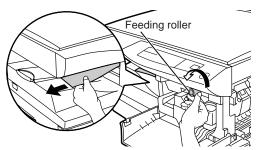
Raise the fusing unit release lever, close the front cover and then close the side cover by pressing the round projections near the side cover open button. The misfeed (8%) indicator will go out and the ready (3) indicator will light up.
