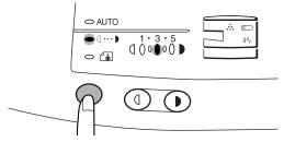
Press and hold down the exposure mode selector key for approximately 5 seconds. The manual (4···•) indicator will go out and the photo (4···•) indicator will begin to blink. The exposure indicator marked "5" will light up, indicating the standard toner mode is active.
