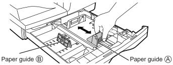
**5** Fan the copy paper and insert it into the tray. Make sure the edges go under the corner hooks.
