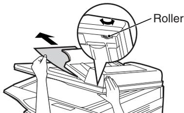
With the RSPF, pull out the reversing tray to remove the misfed original.
