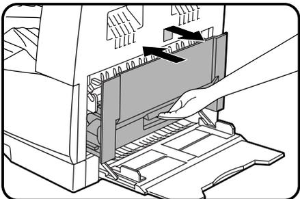
**2** Lift slightly on the side cover and slide the cover out until it stops. Close the side cover by pressing the handle on the cover.
