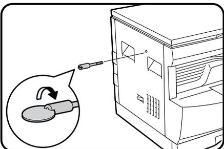
**7** Use a coin (or suitable object) to attach to the left side of the copier the screw that has been stored in the front of the paper tray.
