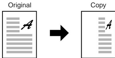
The XY ZOOM feature allows the horizontal and vertical copy ratios to be changed independently.
