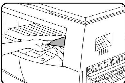
**2** If the misfed paper cannot be removed by the previous step but is visible in the paper output area, remove the paper by pulling it into the paper output area.
