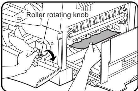
**2** Carefully remove the misfed paper. Turn the roller rotating knob in the direction of the arrow to assist in removing it.
