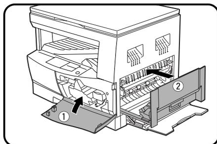
**7** Close the front cover by pushing both sides with your hands and then close the side cover by pressing the handle on the cover. The
