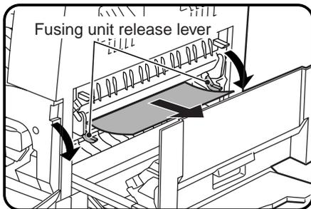
**3** Carefully remove the misfed paper. Lower the fusing unit release levers to allow easier removal. Return the release levers to their operating positions.
