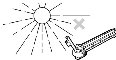
**Store spare supplies such as drum cartridges and TD cartridges in a dark place without removing from the package before use.** If they are exposed to direct sunlight, poor copies may result.
