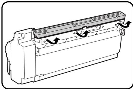
**5** Remove the protective cover from the TD cartridge by unlatching three cover hooks from the holes on the cartridge and then pulling the cover in the direction indicated by the arrow in the illustration.
