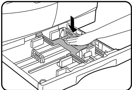
**2** Push the pressure plate down until it locks in place.
