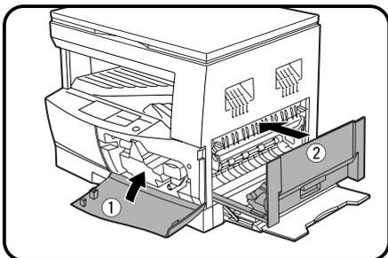
**4** Close the front cover by pushing both sides with your hands and then close the side cover by pressing the handle on the cover.
