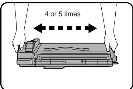
**4** Remove the new TD cartridge from the bag. Hold the cartridge on both sides and shake it horizontally four or five times.
