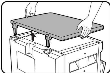
The platen cover can be removed to allow copying of bulky objects. To remove it, simply lift the platen cover straight up.
