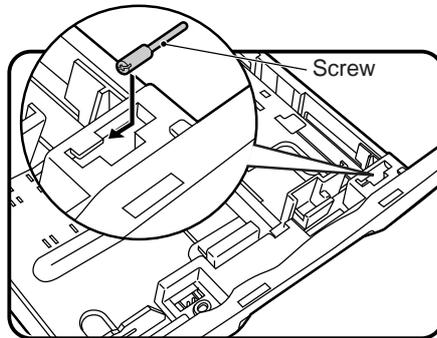
**6 Store the pressure plate lock which has been removed in step 5 and the screw which has been removed in step 2 in the front of the paper tray.**
