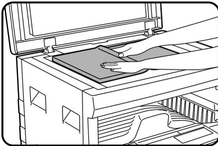
**1** Place the originals on the original table with the center of the two pages aligned with the paper size index (☐ 8½). Close the platen cover.
