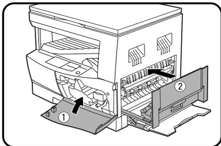
**3** Close the front cover by pushing both sides with your hands and then close the side cover by pressing the handle on the cover.
