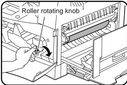
**2** Turn the roller rotating knob in the direction of the arrow.
