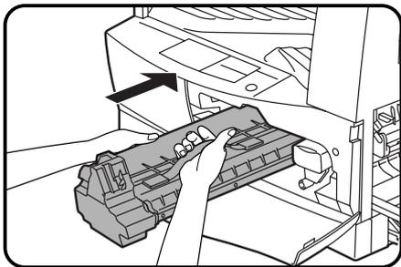
**6** Gently insert the TD cartridge along the guides until it locks in place.
