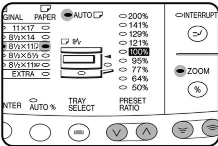
**5** Use the PRESET RATIO selector (  $\nabla$  ,  $\wedge$  ) keys and zoom (  $\odot$  ,  $\otimes$  ) keys to change the copy ratio in the horizontal direction in a similar manner as for the vertical direction.
