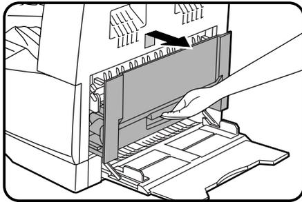
**1** Open the bypass tray. Lift slightly on the side cover and slide the cover out until it stops.
