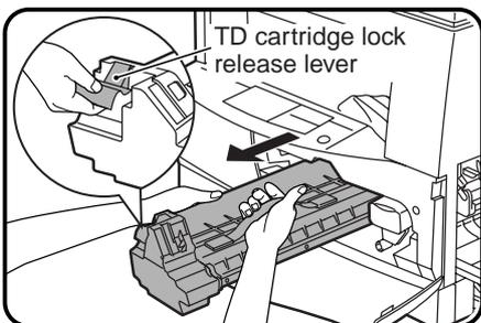
**3** Lift the TD cartridge lock release lever and pull the cartridge out until the green strap handle can be grasped by the right hand. Lift the cartridge by the handle while supporting it with the left hand at the green label position to remove it.
