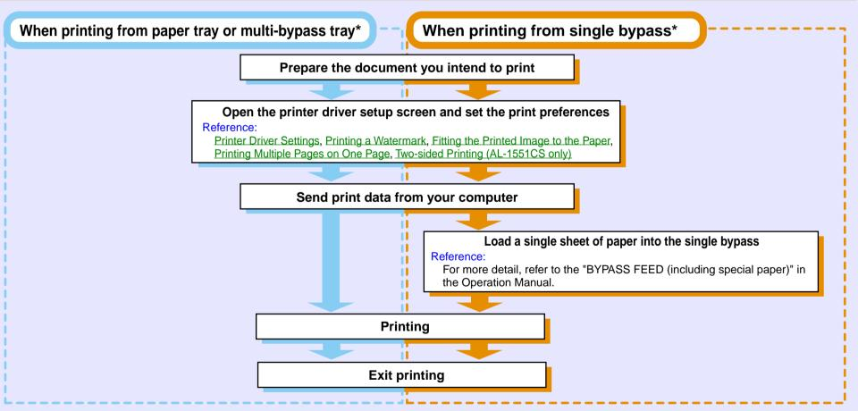
\* The multi-bypass tray can be used on the AL-1551CS, and the single bypass can be used on the AL-1530CS/1540CS. For the procedures for loading paper in each type of tray, see "LOADING PAPER" in the Operation Manual.
