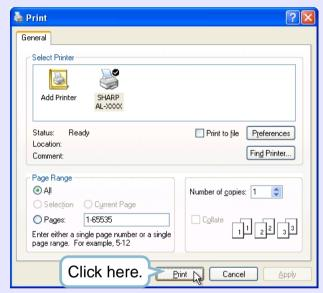
Printing starts according to your preferences. If you are using the single bypass (AL-1530CS/ 1540CS), wait until the single bypass indicator blinks after "P" blinks in the unit display, and insert the sheet of paper in the single bypass.
