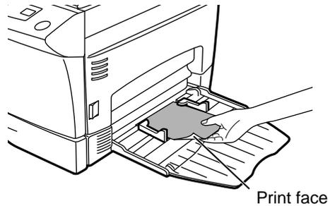
**4** Press the tray select (⊞) key to select the bypass tray. Set the number of copies if using standard copy paper. Press the print (⊞) key.
