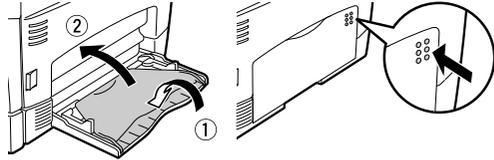
**3** Set the paper guides to the copy paper width. Insert the copy paper (print face down) all the way into the bypass tray.
