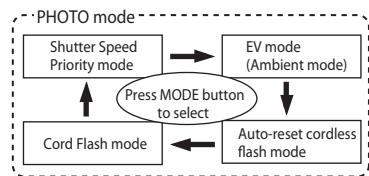
Hold ISO button, and press MODE button to return to the previous Measuring / Setting mode.
