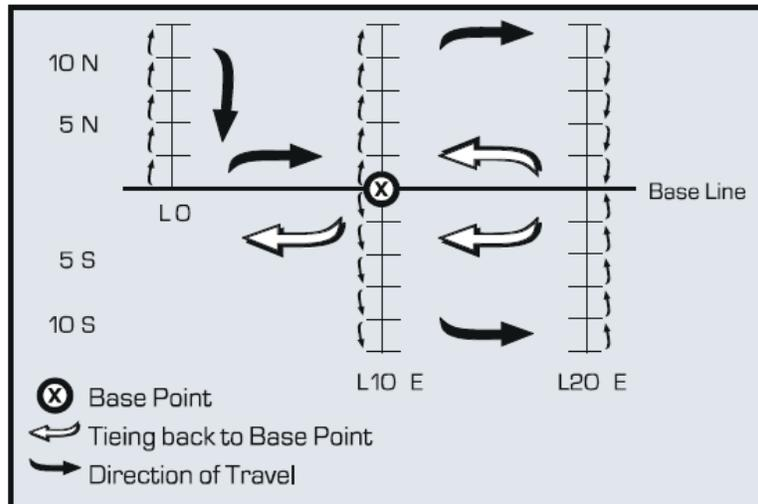
Typical tie-point method in loop mode survey
