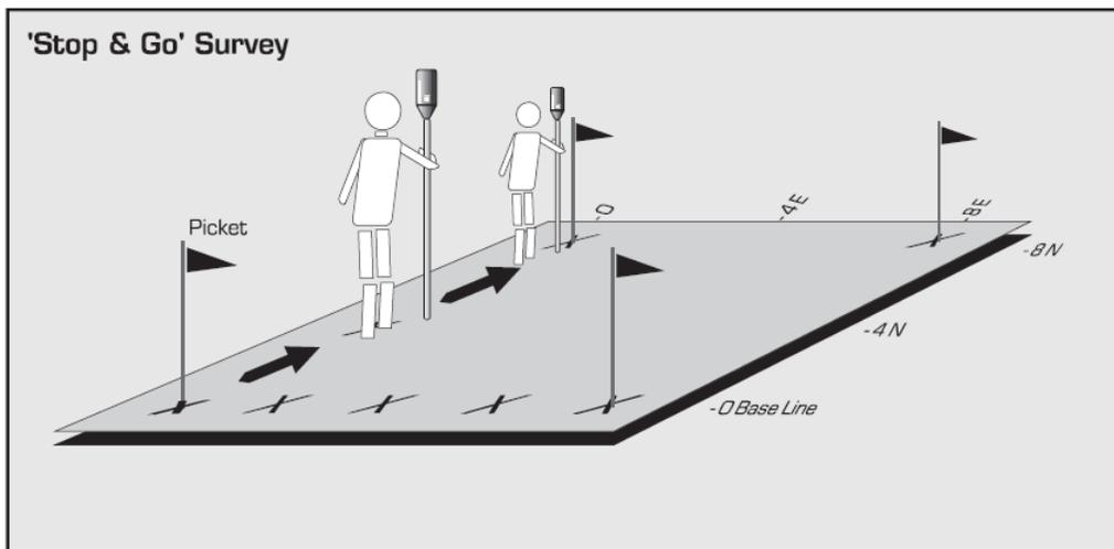
Set-up for a Stop-and-Go survey
