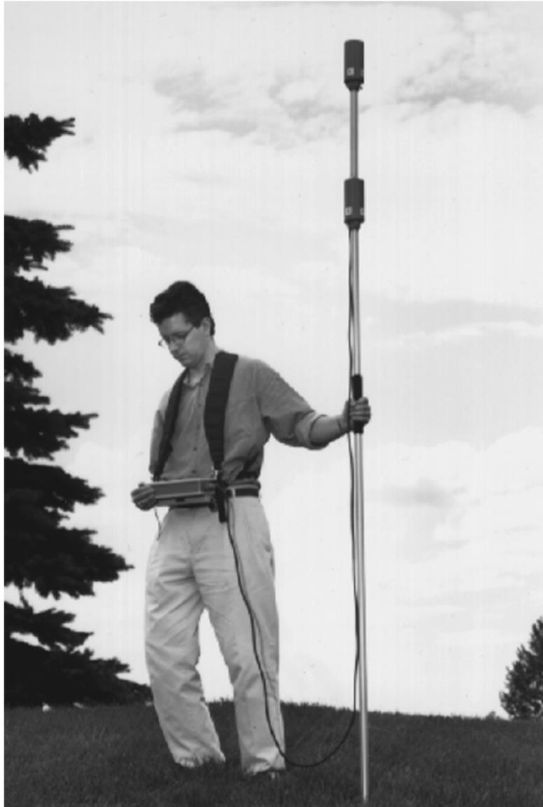
Typical gradiometer configuration
