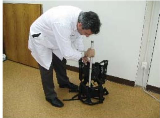
2. If you are using the GPS antenna, insert the GPS antenna mount on top of the previous staff section, as illustrated.
