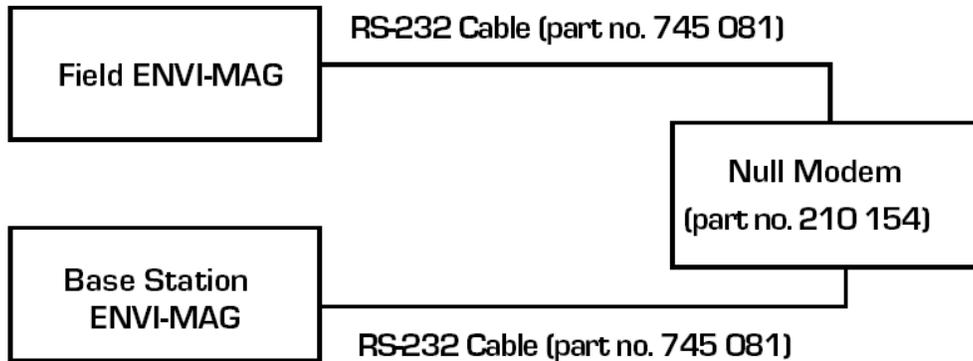
Connections for the Base-station correction
