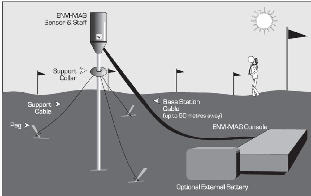
Typical base-station sensor setup
