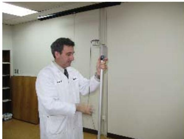
3. Insert another staff section in order to clamp the GPS antenna mount between two staff sections as illustrated.
