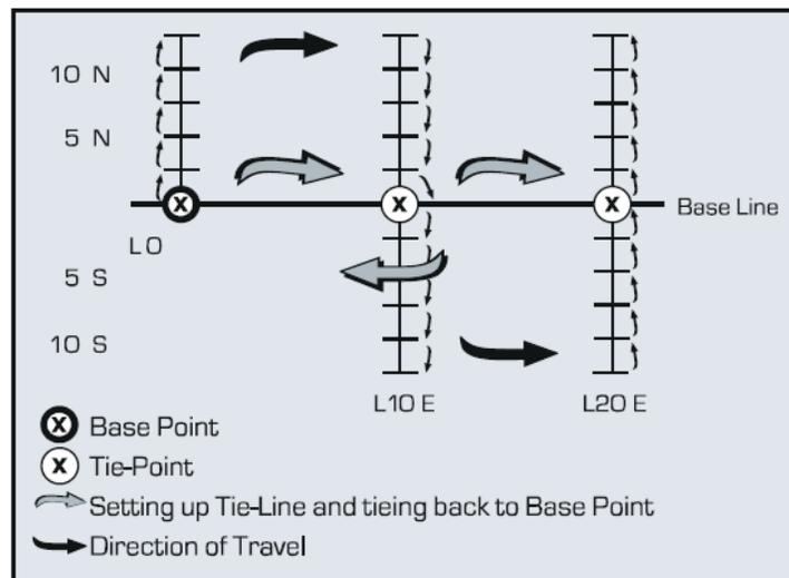
Typical tie-point method in line survey
