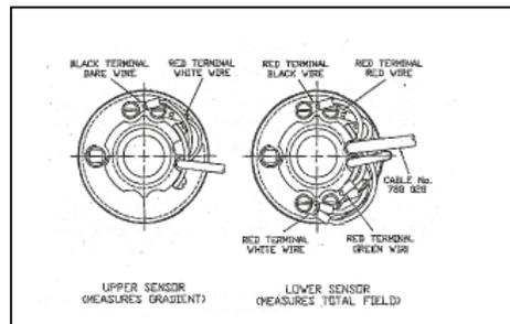
Gradiometer sensor cabling
