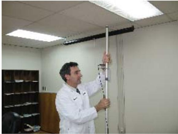
4. Insert the magnetometer sensor on the top section as illustrated.
