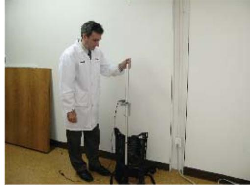
4. Insert the magnetometer sensor at the top of the second staff section, as illustrated.
