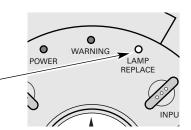
This indicator lights yellow when the life of the projection lamp draws to an end.
