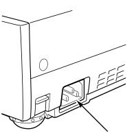
Connect the AC Power Cord (supplied) to the projector. The AC outlet must be near this equipment and must be easily accessible.
