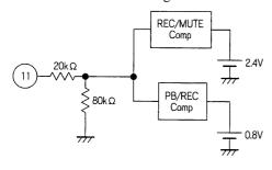
GND < pin 11 level - DC < 1.0 V: PB mode 1.0 V < pin 11 level - DC < 3.0 V: REC mode, REC-MUTE 3.0 V < pin 11 level - DC < 5.0 V: REC mode
