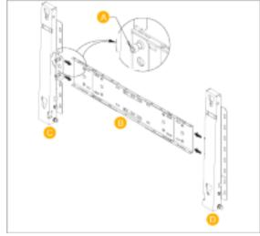
When done, mount the wall bracket on the wall.
