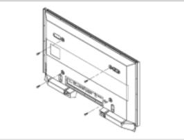
2. Insert the screw B into the plastic hanger.
