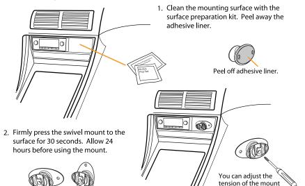
If you need to remove the mount, carefully lift the adhesive pad with your fingers or a spoon. Warming with a hair dryer for several minutes will help soften the adhesive.
