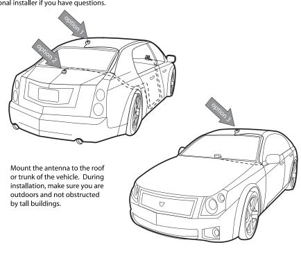
Warning: Failure to properly install the antenna may result in injury to yourself or to others if it becomes detached during an accident.
