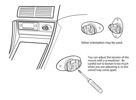
If you need to remove the mount, carefully lift the adhesive pad with your fingers or a spoon. Warming with a hair dryer for several minutes will help soften the adhesive.
