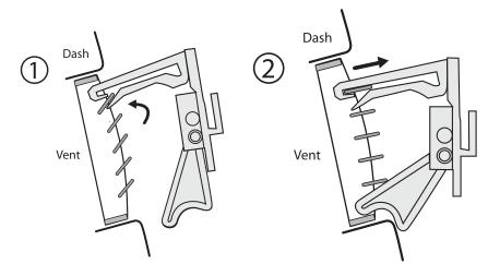
To remove the vent mount, push it into the vent and lift upwards slightly to release the mount's hooks from the vent vane.
