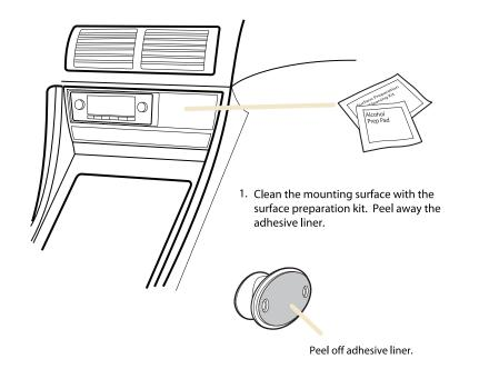
2. Firmly press the swivel mount to the surface for 30 seconds. Allow 24 hours before using the mount.
